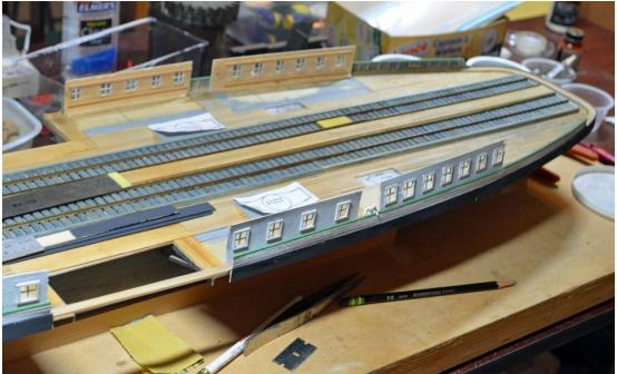
**No. 4: 3** The caps were two 1/16" square planks to accommodate the curves. The walkway planking in place running across the Wheel Box is fitted and lifted off and set aside until the comletion of the Box.
