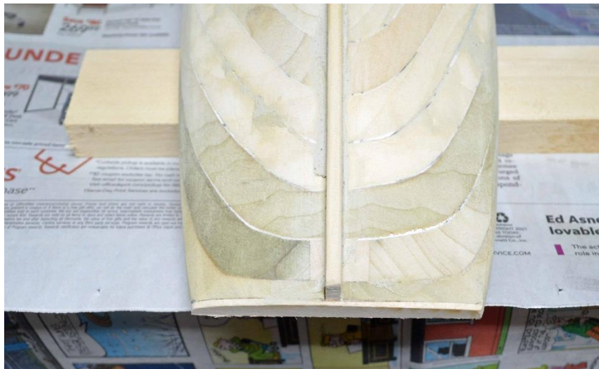
No. 2: 5 This is the docking end of the ferry's hull set to receive "tail gate" beam assembly. Note the 1/16" basswood "cap". I added that piece to cover the grain of poplar and to assure I had a smooth gluing surface for this assembly.
