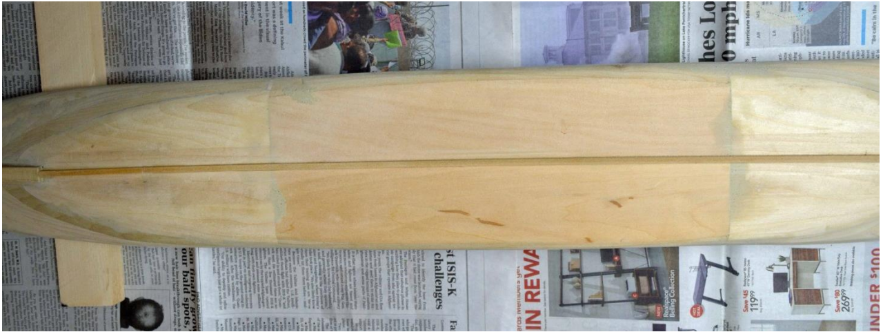
No. 8: Note the keel (1/8" x 1/8" basswood) down the centerline..
